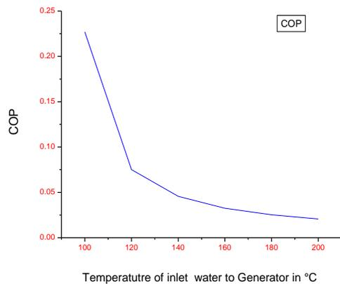
Figure 3: Variations of COP with inlet water temperature to Generator ( $T_{11}$ )
