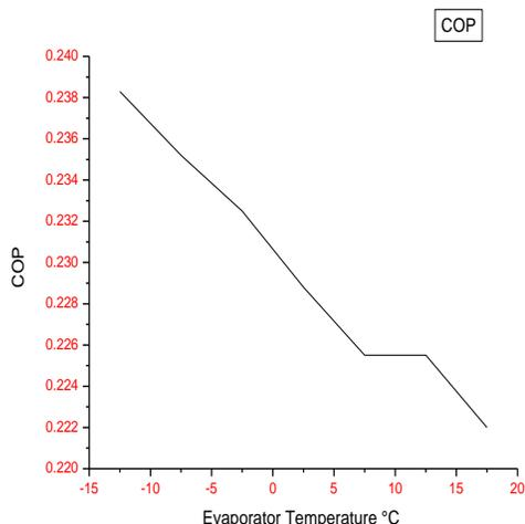
Figure 5: Variations of COP with Evaporator Temperature
